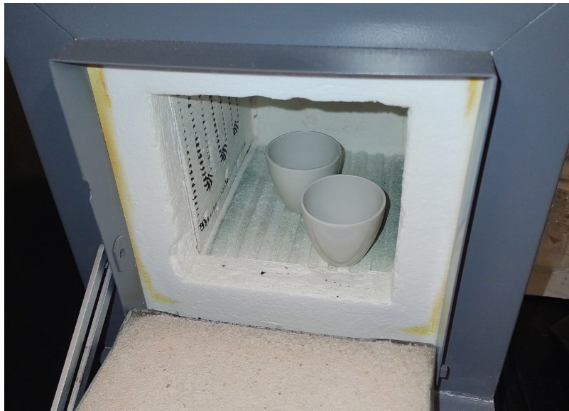
Figure 24. Soil samples in the oven. Loss on ignition is a technique where soil samples are weighted then heated to high temperatures and weighted again. The high temperature will oxidize any organic matter in the sample, and the difference in weight will be used to calculate the amount of organic matter. Source of the image USGS – NMWSC 2021.
